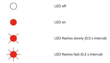
During the charging process, the capacity is indicated by the lighting and flashing of the LEDs on the battery as follows:
