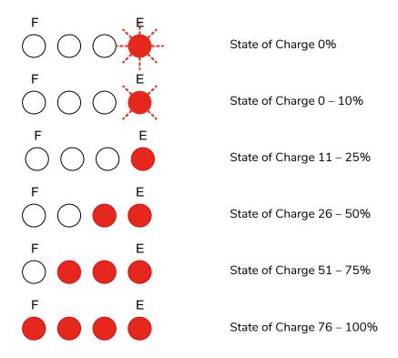
By pressing the button on the battery for a longer time, further information can be displayed.
